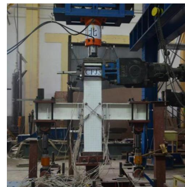
Fig. 3 Test setup of the composite joints under cyclic loading
