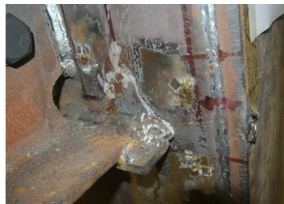
(b) Weld cracking and tearing of skin plate
