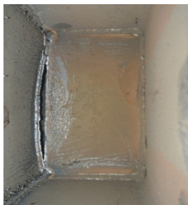
(a) Weld cracking between the skin plate and diaphragm
