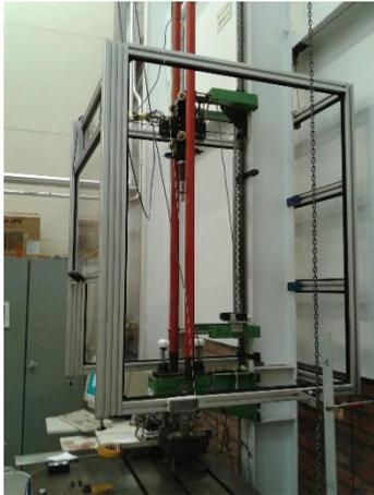
(a) Tower of drop weight apparatus
