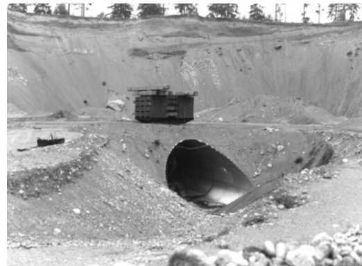
Fig. 1 Enköping pipe arch, loading to failure test. Steel weights were used to increase the load on the axle simulating the live load
