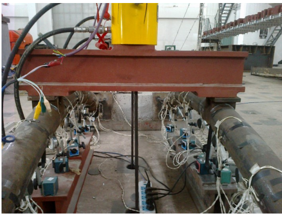
Fig. 3 Load distributing girder
