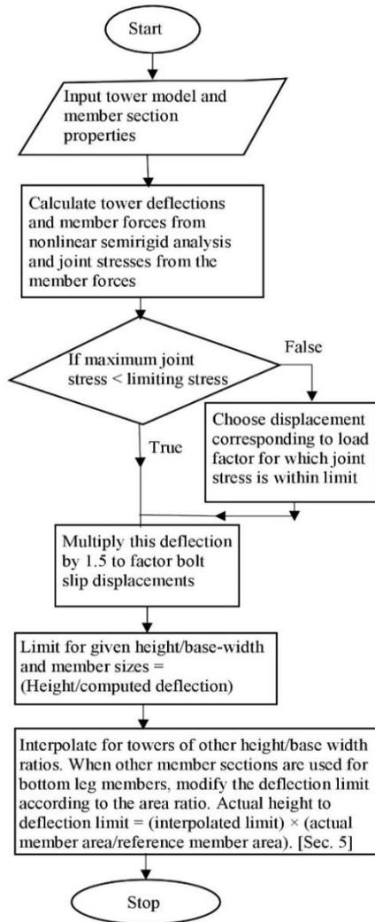
Fig. 7 Height to deflection limit determination procedure proposed in this study
