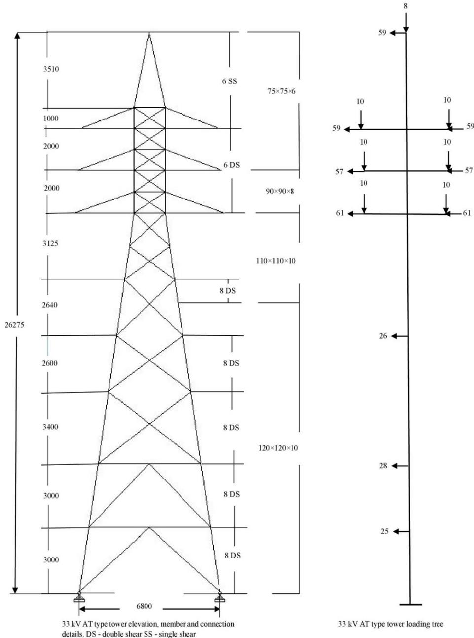
Fig. 1 33 kV AT Type tower elevation and loading tree (units: kN, mm)
