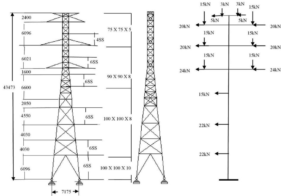
Fig. 6 240 kV K-type tower elevation and loading tree. DS - double shear SS - single shear (units: kN, mm)
