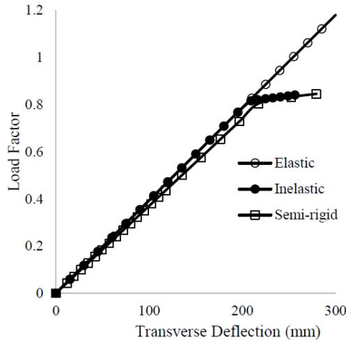
Fig. 4 Load-deflection of AT-type tower
