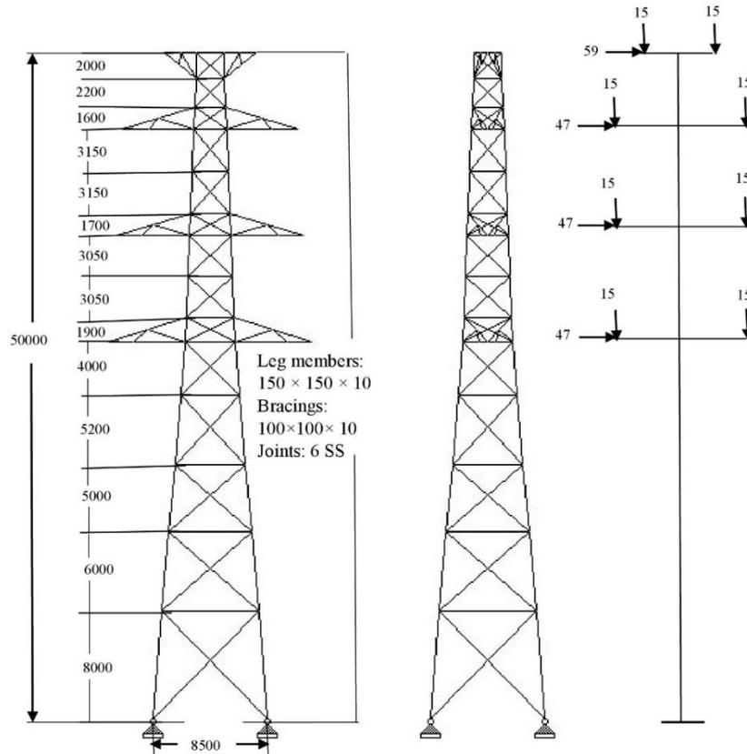
Fig. 2 Double circuit tower elevation and loading tree (units: kN, mm)
