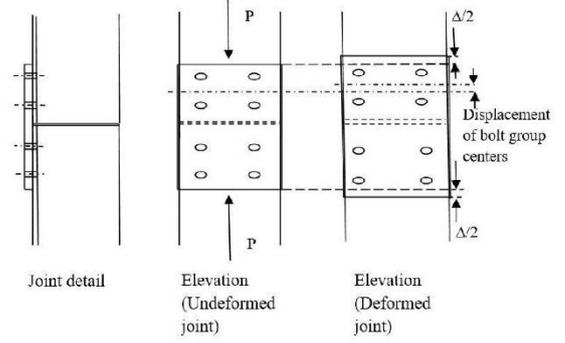
Fig. 3 Cover plate axial deformations joining leg members
