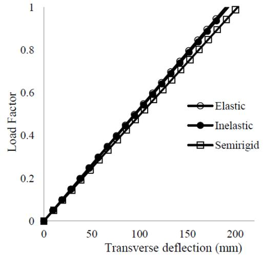
Fig. 5 Load-deflection of double circuit tower
