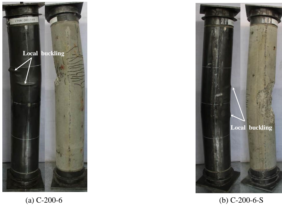
Fig. 6 Failure modes of slender columns ( L/D = 6 )
