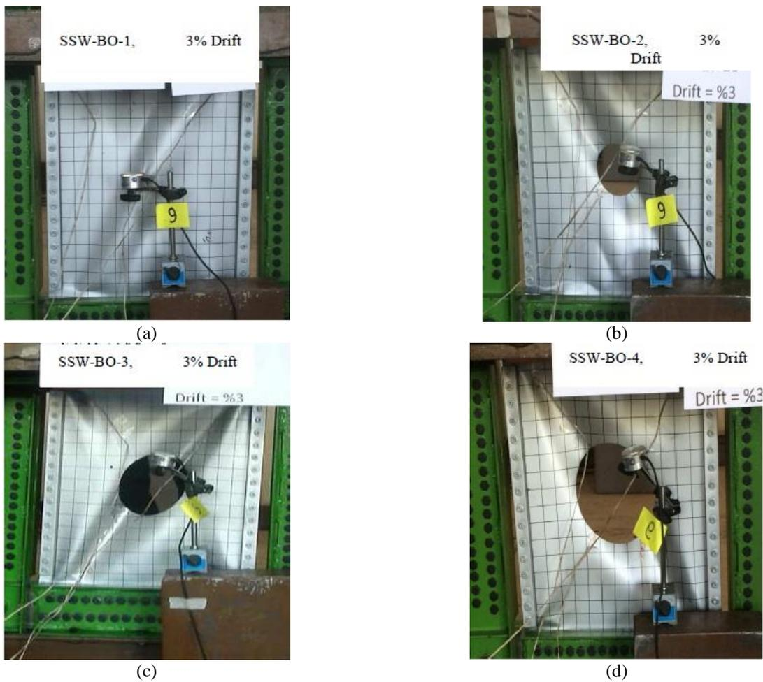
Fig. 11 Out of plane deformation at 3% drift: (a) SSW-BO-1, (b) SSW-BO-2, (c) SSW-BO-3 and (d) SSW-BO-4
