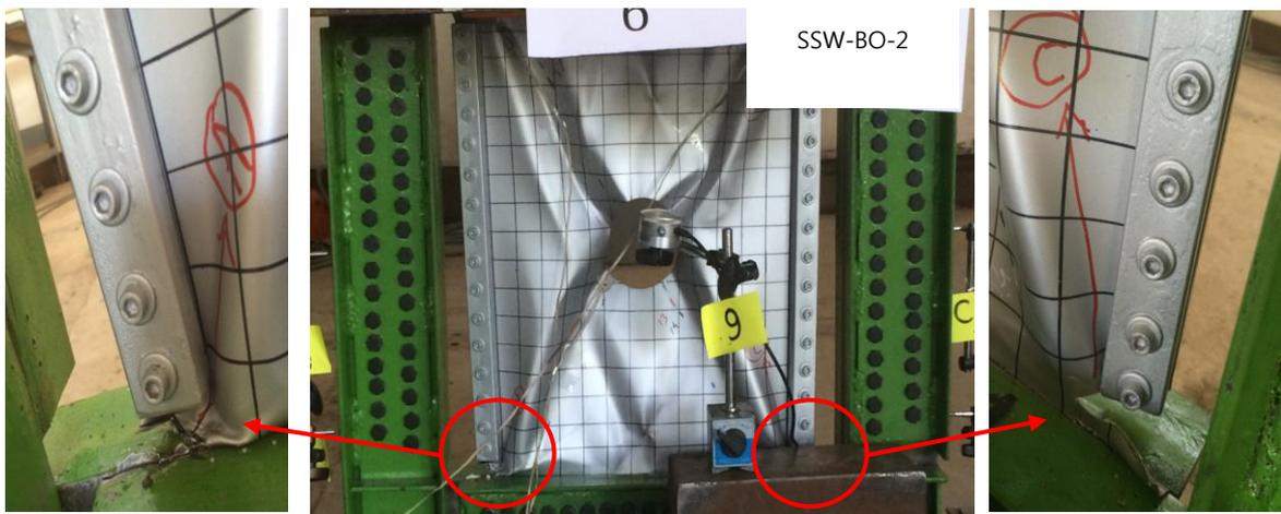
Fig. 8 Local tears at the lower corners of SSW-BO-2
