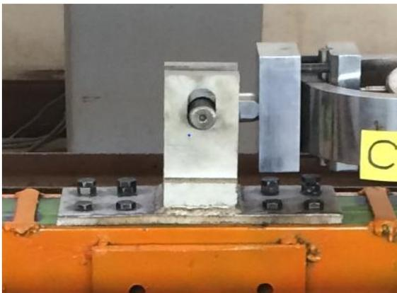
Fig. 4 Pin connection of hydraulic jack to top of the specimens
