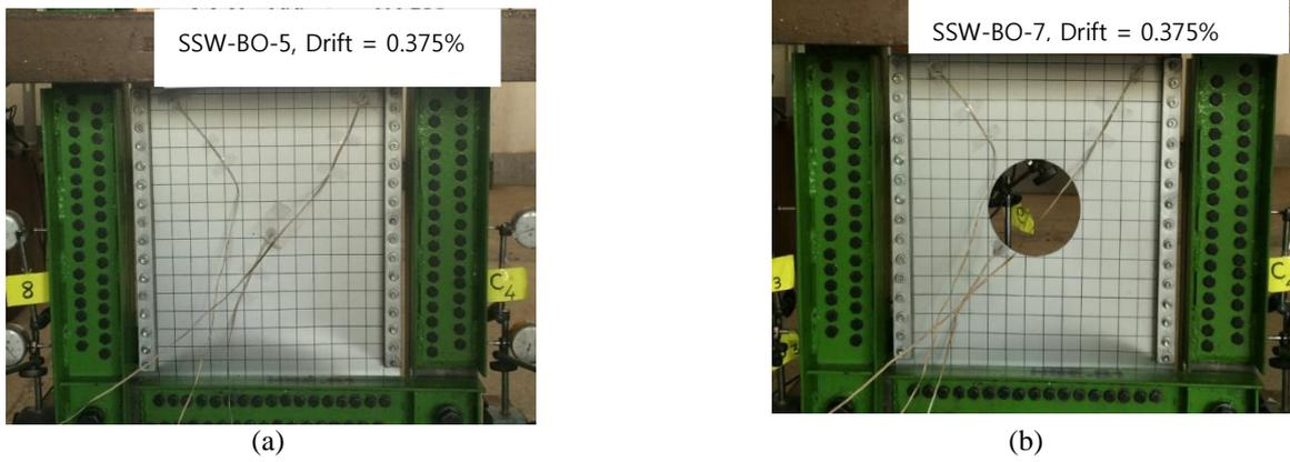
Fig. 10 Out of plane buckling at the lower corners at early stage of loading: (a) SSW-BO-5 and (b) SSW-BO-7
