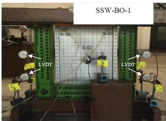
Fig. 5 Installation place of the transducers and the strain gauges in the SSW-BO-1 specimen
