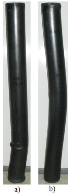
Fig. 11 Failure modes of the specimens with L/D = 10.5 . (a) LWC-114.3-3.38-10.5, and (b) SCC-114.3-3.38-10.5
