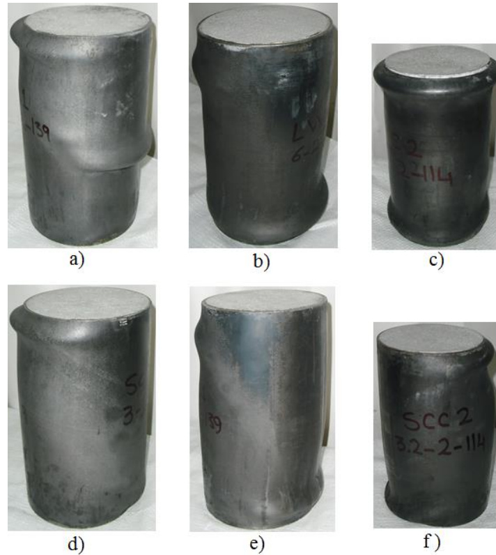
Fig. 8 Failure modes of the specimens with L/D = 2 . (a) LWC-139.7-3.30-2, (b) LWC-139.7-5.87-2, (c) LWC-114.3-3.38-2, (d) SCC-139.7-3.30-2, (e) SCC-139.7-5.87-2 and (f) SCC-114.3-3.38-2
