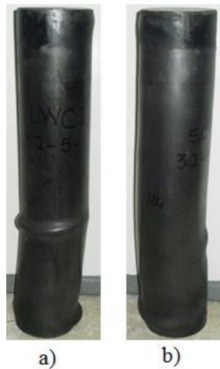
Fig. 9 Failure modes of the specimens with L/D = 5 . (a) LWC-114.3-3.38-5 and (b) SCC-114.3-3.38-5
