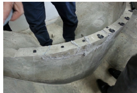
Fig. 12 Repair process of arch dam with epoxy mortar
