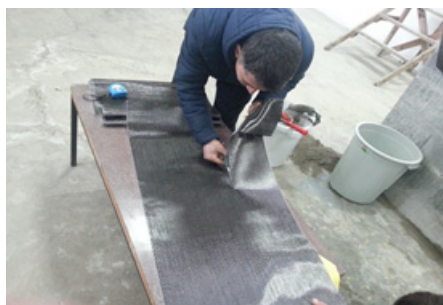
(b) Application of MBT-MBrace®Adesivo to the body surface
