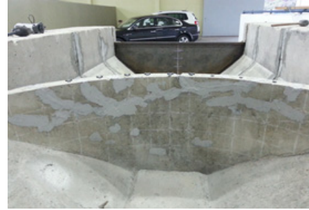
(e) Application of structural repair mortar on the surface of dam arc
