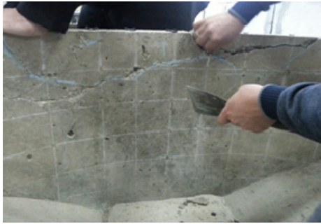
(a) Removal of the damaged concrete pieces
