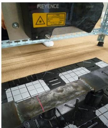
(b) Thickness measurement by 3D measuring device
