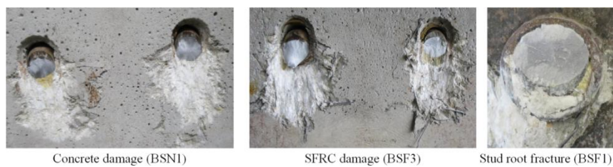
(a) Static push-out failure (stud fracture with local concrete or SFRC damage)
