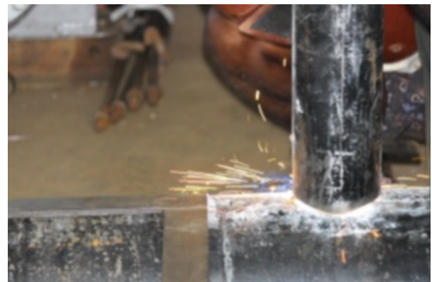
Fig. 2 Tube connection and tack welding
