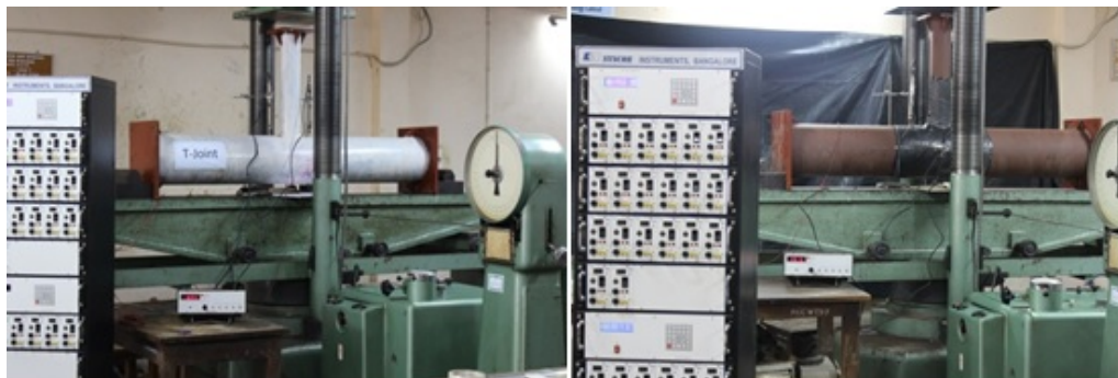
Fig. 8 Specimen arrangement on compression and bending testing machine
