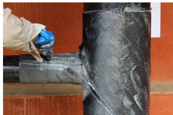
Fig. 6 Wrapping of CFRP on Tubular joint
