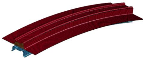
Fig. 6 Deep drawing analysis performed for the bumper beam and the crash box
