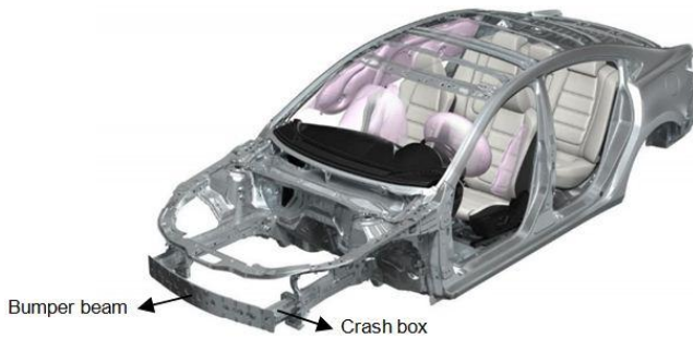
Fig. 1 Body structure and energy absorption components of a vehicle (URL 2016a)
