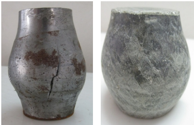
Fig. 12 Failure mode of STCC specimen (left) and concrete core separated from the steel tube after failure point (right)
