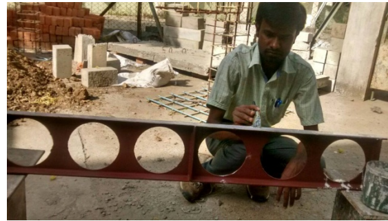
Fig. 2 White washing of the test specimen
