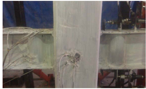
(b) Local buckling at 5% story drift
