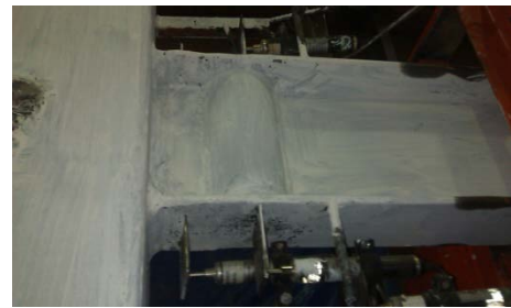
(b) The extension of the yielding at 2% story drift
