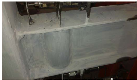
(a) First yielding at the center of the reduced region at 1.5% story drift
