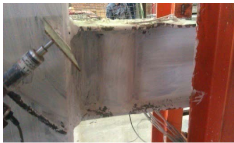
(a) Lateral-torsional buckling in the left beam at 7% story drift
