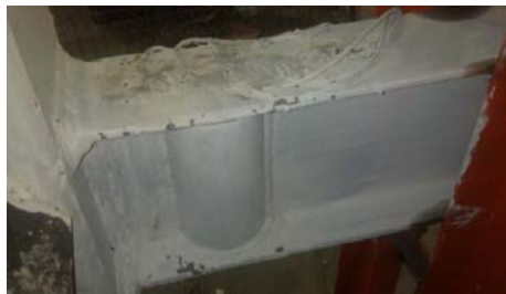
(c) The extension of the yielding at 3% story drift
