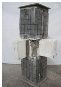
Fig. 5 The failure patterns of the specimens in Group GS
