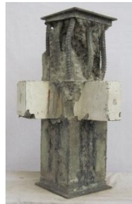
Fig. 5 The failure patterns of the specimens in Group GS
