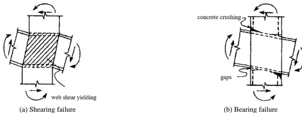
Fig. 13 Failure modes for RCS connections by Sheikh *et al.* (1989)
