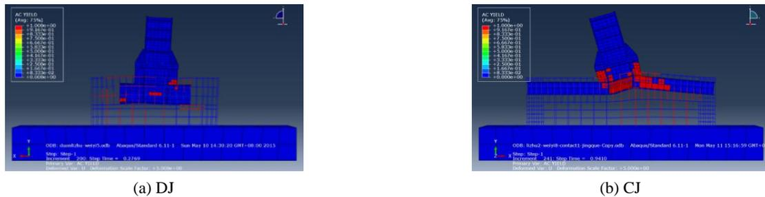
Fig. 5 Predicted stress distribution in steel members and reinforcement at failure of specimens
