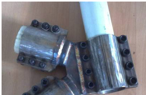
Fig. 2 Composite tube connection based on PTTC
