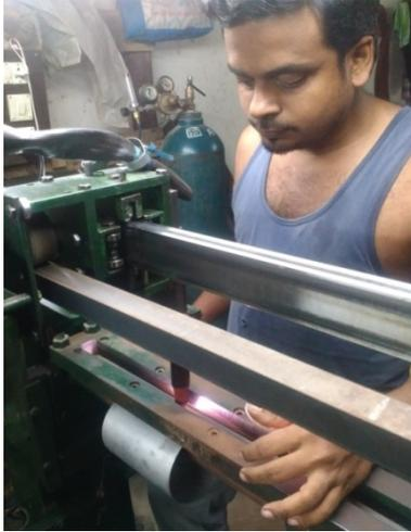
Fig. 1 Fabrication of specimen by TIG welding
