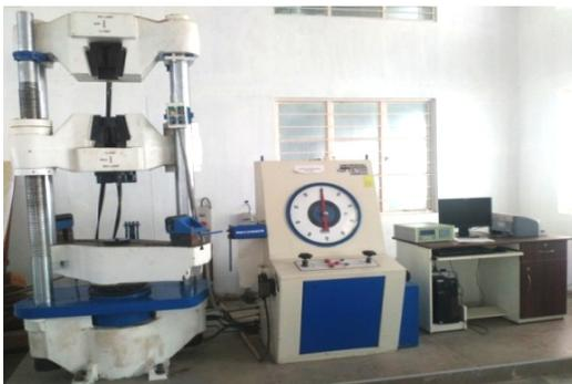
Fig. 4 Servo controlled Universal Testing Machine
