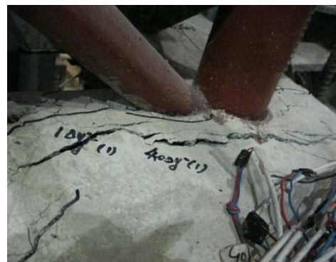
Fig. 7 Concrete flange transverse fracture
