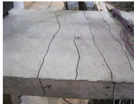
Fig. 5 Cracks developing of the concrete flange
