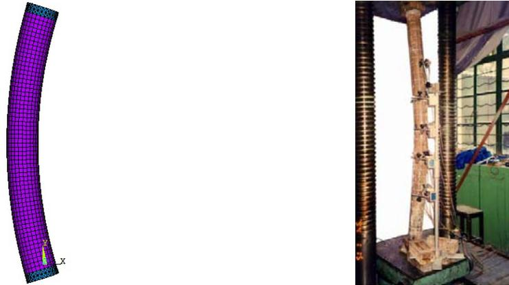
Fig. 6 General view of the failure mode of verification model vs. Tested specimen
