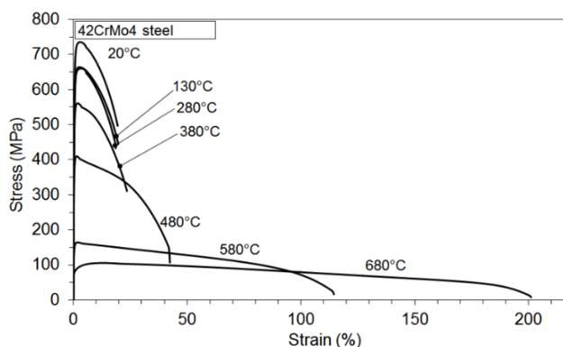
Fig. 1 Engineering stress-strain diagrams: 42CrMo4 steel
