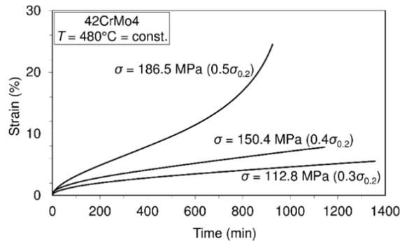
Fig. 3 Creep behavior of 42CrMo4 steel at 480°C
