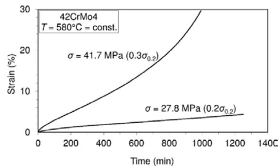
Fig. 4 Creep behavior of 42CrMo4 steel at 580°C
