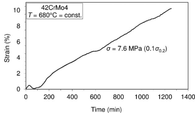
Fig. 5 Creep behavior of 42CrMo4 steel at 680°C
