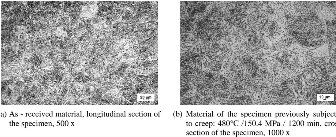
Fig. 7 Steel 42CrMo4: optical micrographs, 4% nital
