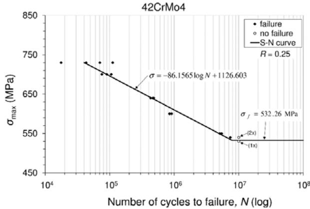
Fig. 8 Fatigue tests data and approximated  $S - N$  curve in finite and infinite fatigue regions at room temperature and stress ratio of  $R = 0.25$
