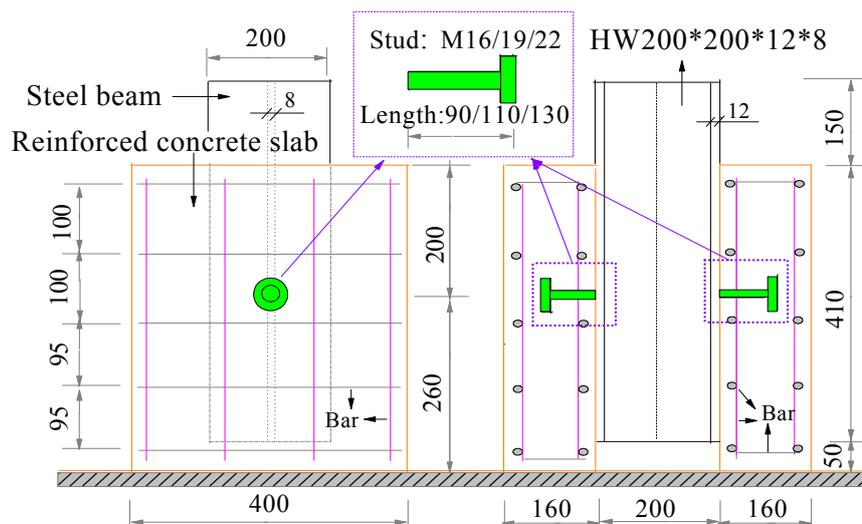
Fig. 1 Size of push-out test specimen: front view (left); side view (right)
