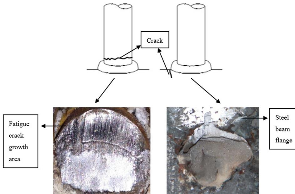
Fig. 4 Fatigue failure modes of fatigue push-out tests: Fatigue failure of stud (Left); Tearing off the base metal (right)
