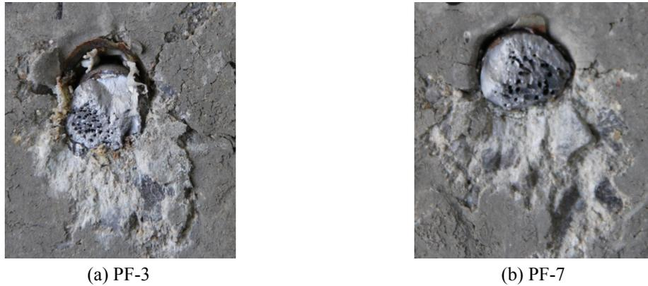
Fig. 5 Welding defects in PF-3 and PF-7
