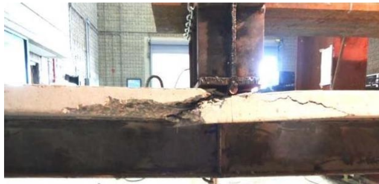
Fig. 14 Shear-compression failure at mid-span region
