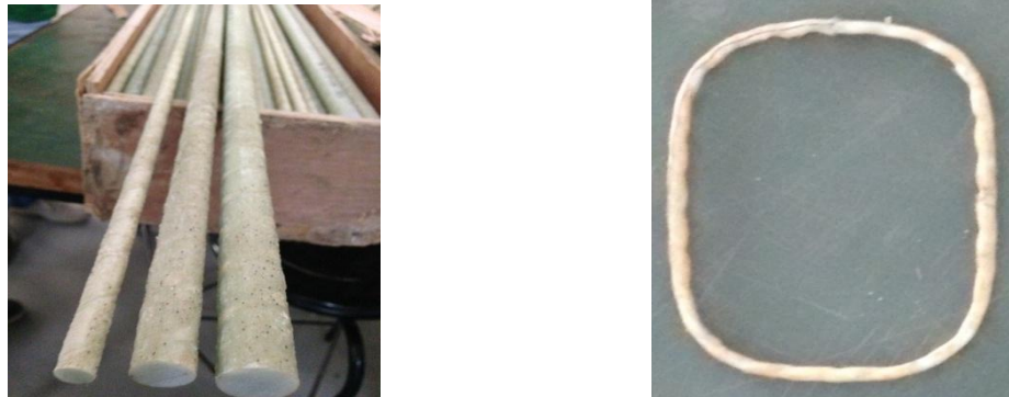
Fig. 2 GFRP bars and stirrup
