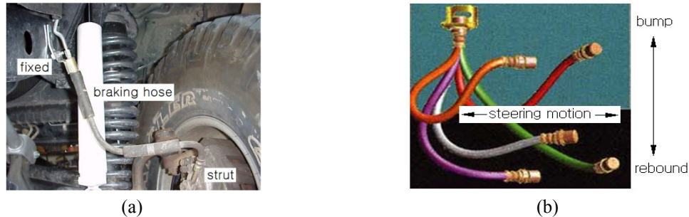
Fig. 1 (a) Braking hose assembled in the front wheel; (b) steering and bump/rebound motions
