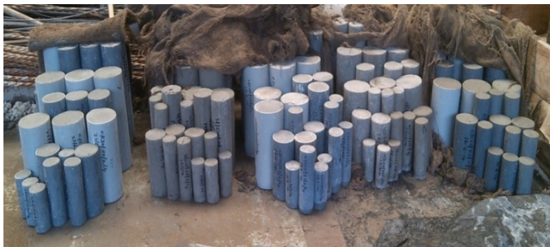
Fig. 2 Samples of stub columns ready for testing
