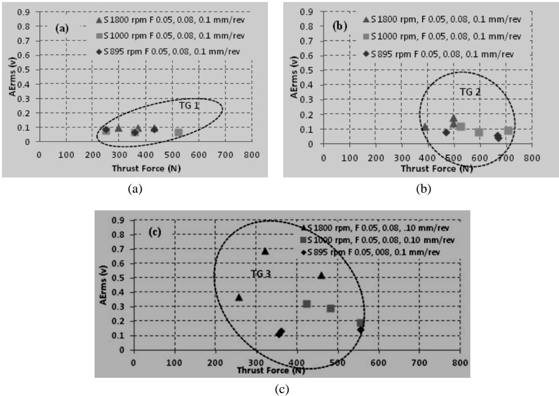
Fig. 8 Influence of AErms value and machining conditions with respect to modified tool geometry: (a) TG1; (b) TG2; (c) TG3
