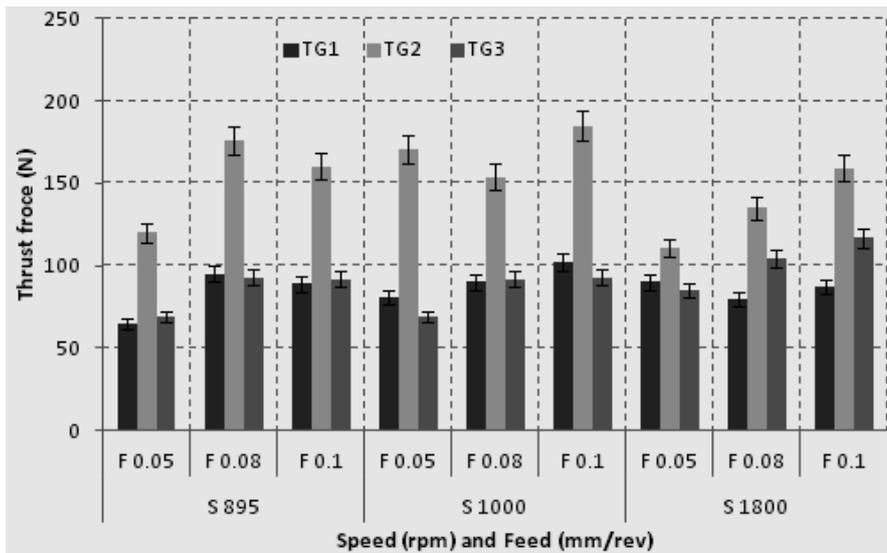
Fig. 5 Thrust force in machining CFRP
