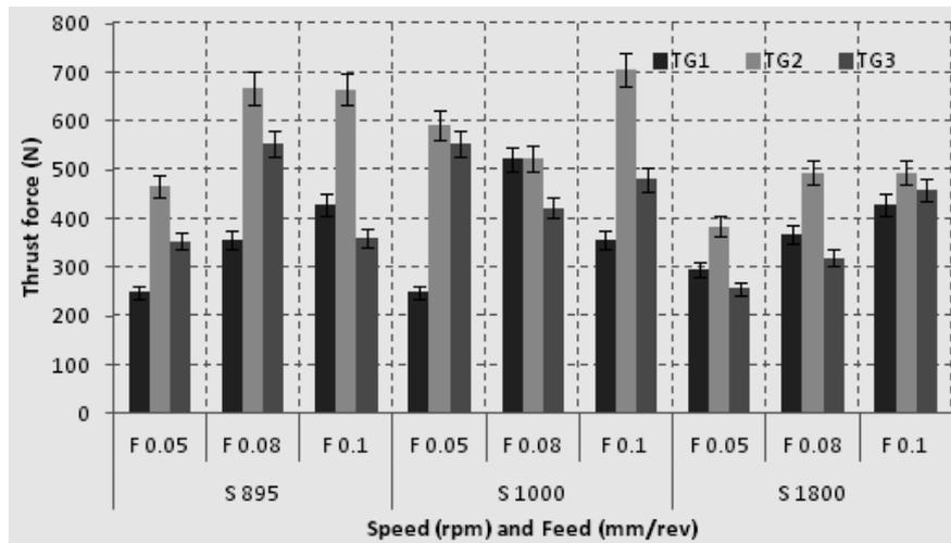
Fig. 6 Thrust force in machining Ti6Al4V
