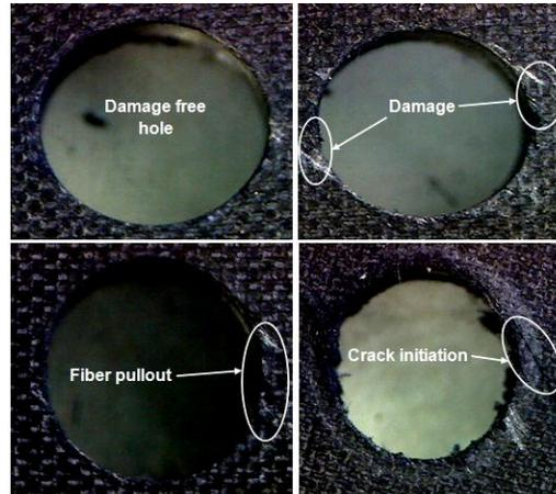
Fig. 9 Delamination in different modes of failure
