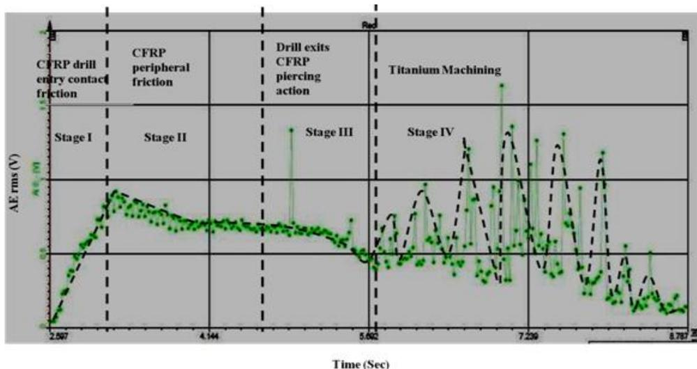
Fig. 3 Stages in drilling of CFRP/Ti6Al4V stack
