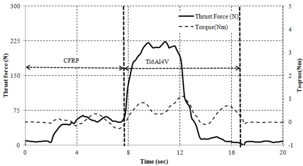
Fig. 4 Thrust force and torque during drilling of CFRP/Ti6Al4V stack
