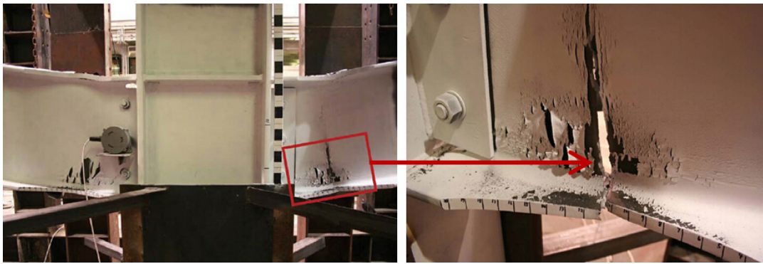
Fig. 6 Failure mode of steel SMF assembly (Sadek et al. 2009, 2013)
