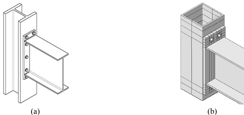
Fig. 1 General end-plate connections to (a) Open section column (Adam and Hamburger 2010); (b) Tubular column
