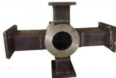
(b) Test specimen with ribbed stiffener
