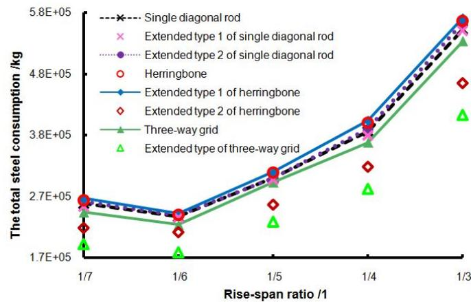
Fig. 27 The total steel consumption of eight cylindrical reticulated shells when span is 80m
