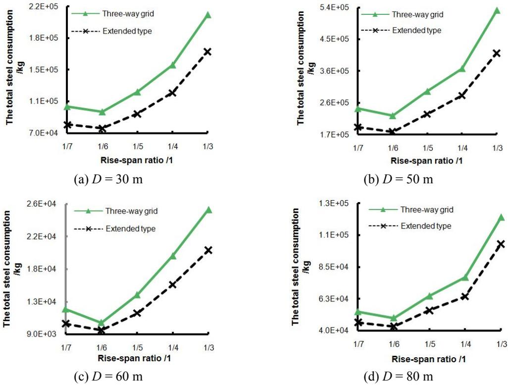
Fig. 23 The total steel consumption for fundamental type and extended type of three-way grid - cylindrical reticulated shell
