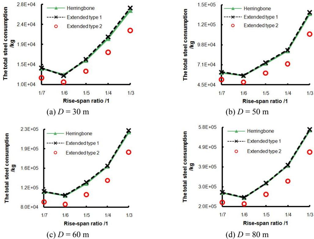
Fig. 22 The total steel consumption for fundamental type and extended types of herringbone - cylindrical reticulated shell
