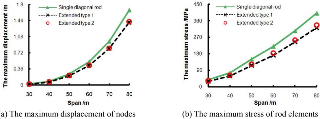
Fig. 15 The results of internal force analysis for single diagonal rod and its extended types
