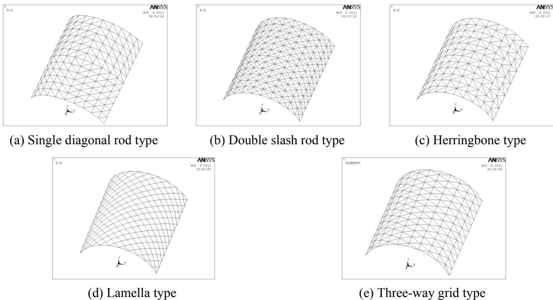
Fig. 3 Five fundamental types of cylindrical reticulated shell
