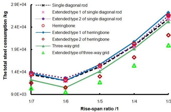
Fig. 24 The total steel consumption of eight cylindrical reticulated shells when span is 30m
