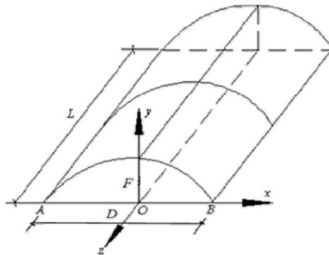
Fig. 2 Structure diagram of cylindrical reticulated shell
