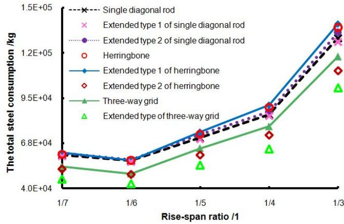
Fig. 25 The total steel consumption of eight cylindrical reticulated shells when span is 50m
