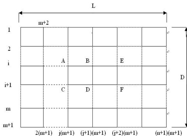
Fig. 7 The nodes distribution of cylindrical reticulated shells
