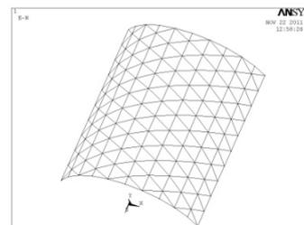
(e) Extended type of three-way grid
