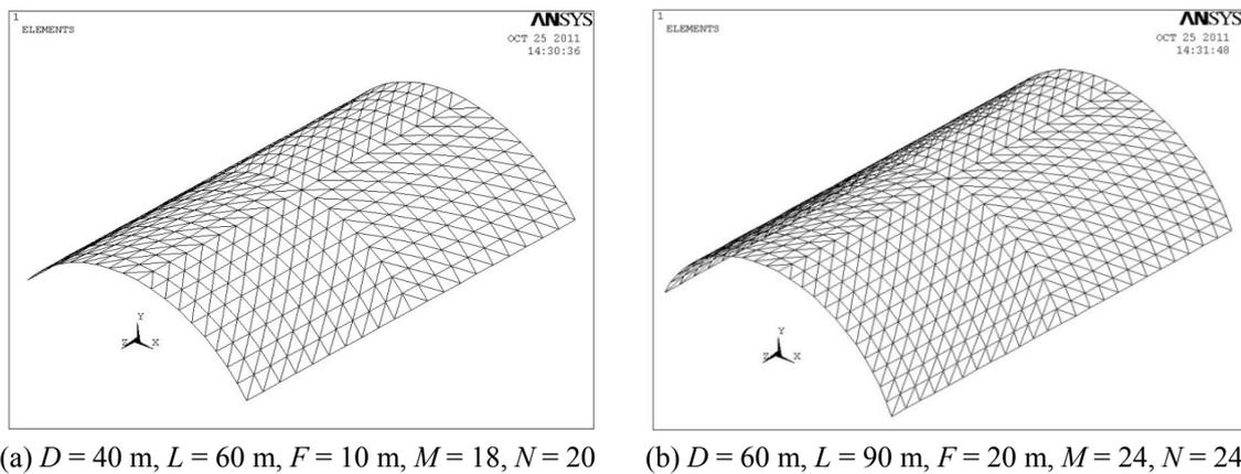
Fig. 8 Extended type 1 of single diagonal rod
