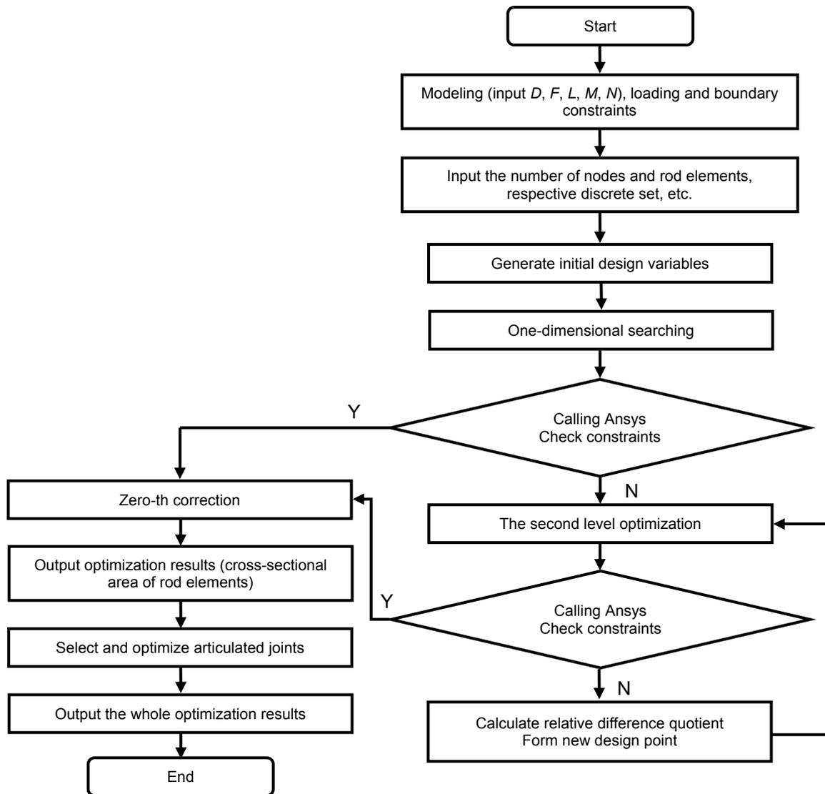
Fig. 20 Cross-section optimization flowchart of cylindrical reticulated shells
