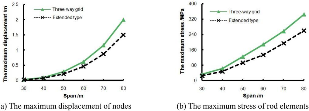
Fig. 17 The results of internal force analysis for three-way grid and its extended type
