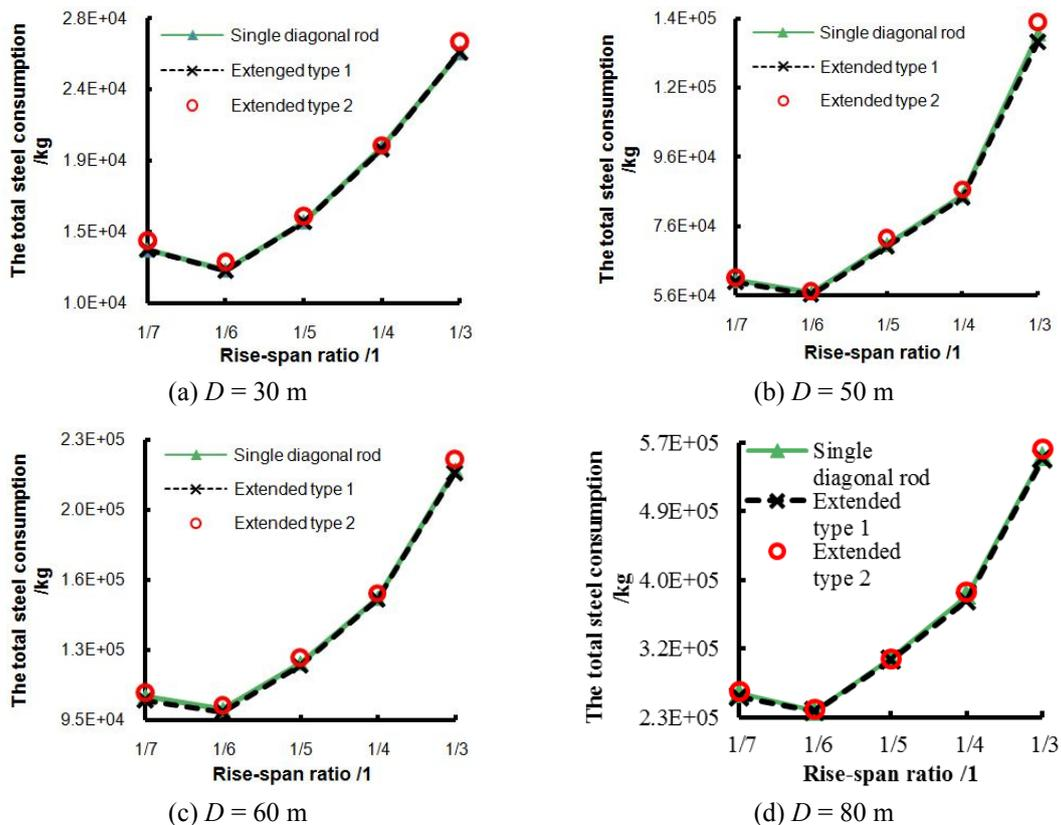
Fig. 21 The total steel consumption for fundamental type and extended types of single diagonal rod - cylindrical reticulated shell
