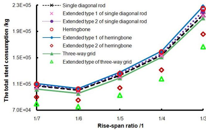
Fig. 26 The total steel consumption of eight cylindrical reticulated shells when span is 60m
