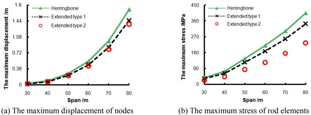
Fig. 16 The results of internal force analysis for herringbone and its extended types
