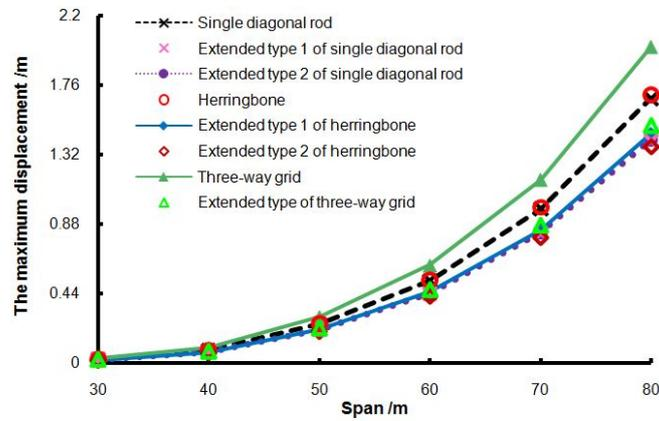
Fig. 18 The maximum displacement of eight cylindrical reticulated shells under different span
