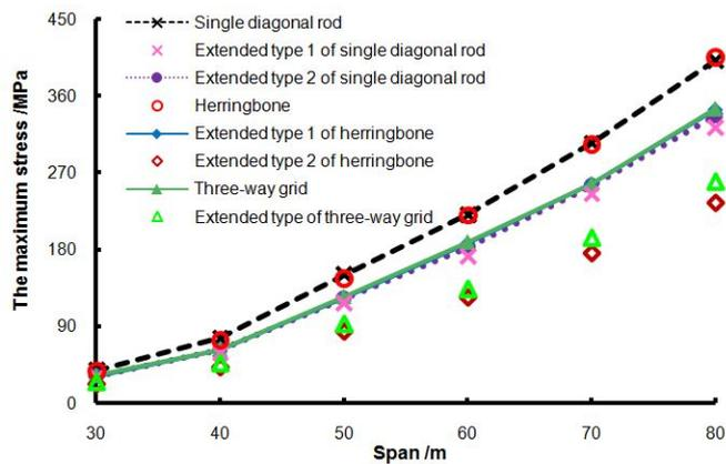
Fig. 19 The maximum stress of eight cylindrical reticulated shells under different span
