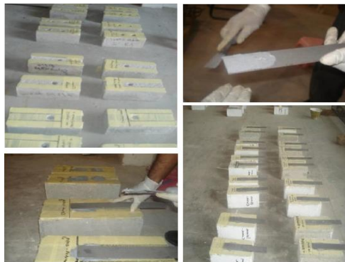
Fig. 6 Steel plates bonded to the concrete prisms for the pull-out test
