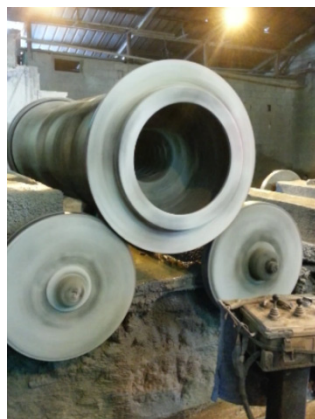
(c) Placing concrete and rotating mold
