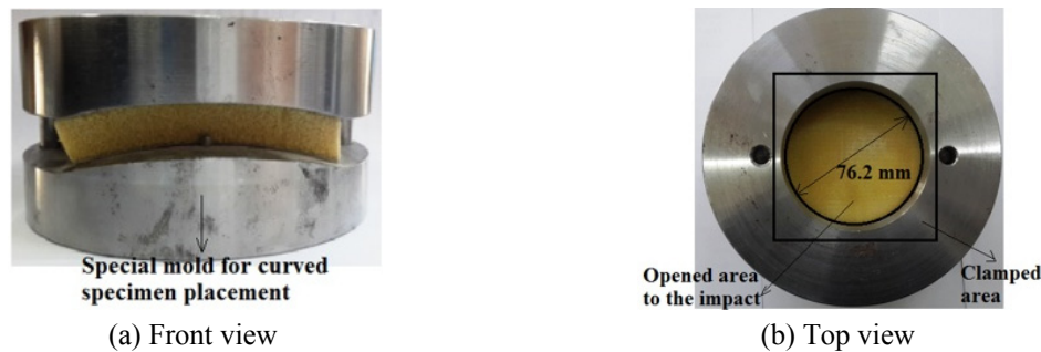
Fig. 4 Photos of clamping apparatus for curved panel
