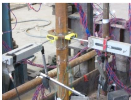
Fig. 4 Arrangement of displacement transducers
