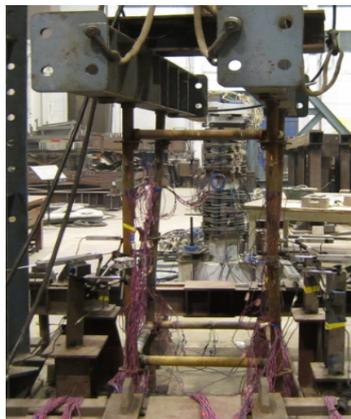
(a) Buckling mode of specimen 1
