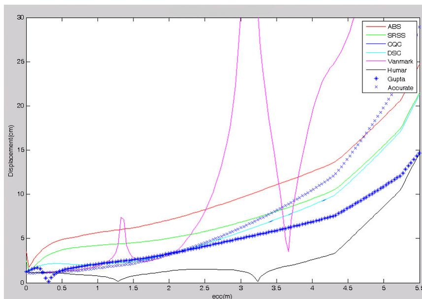
Fig. 4 The lateral displacement relative to structural eccentricity for all methods in the first mode
