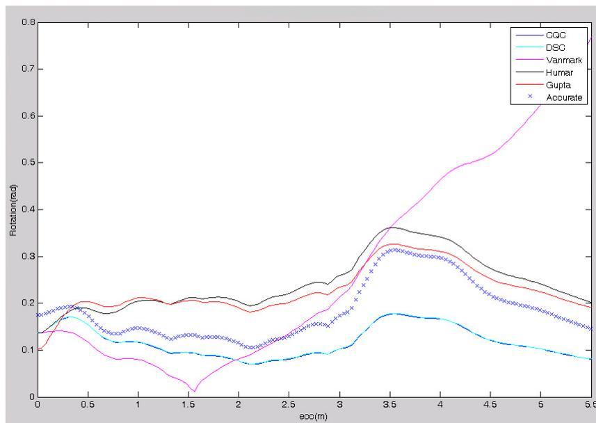
Fig. 6 The lateral displacement relative to structural eccentricity for all methods in the third mode
