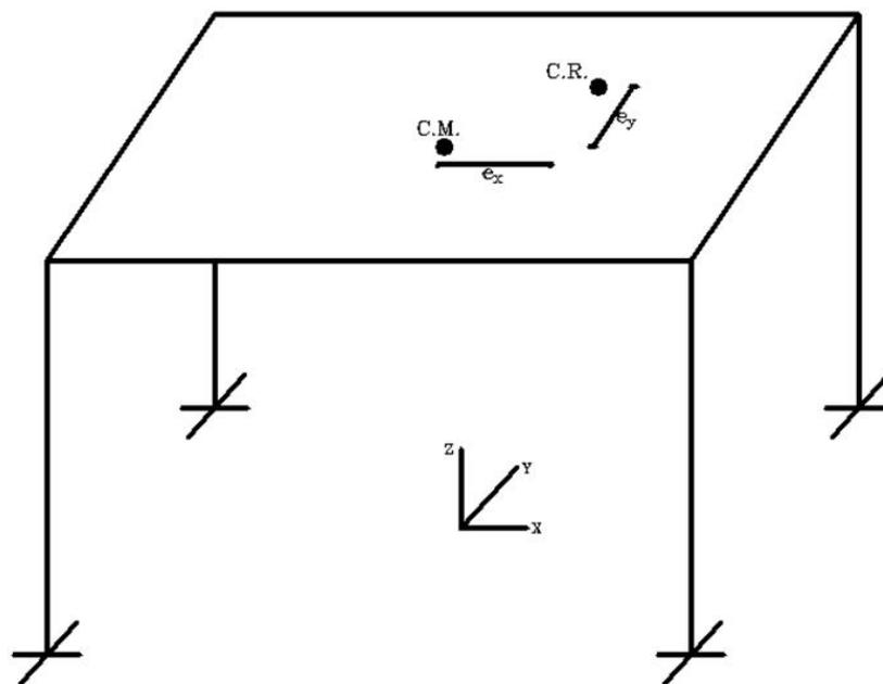
Fig. 1 The center of mass and rigidity in one storey building
