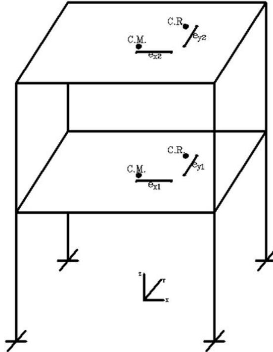
Fig. 2 The center of mass and rigidity in two floors building
