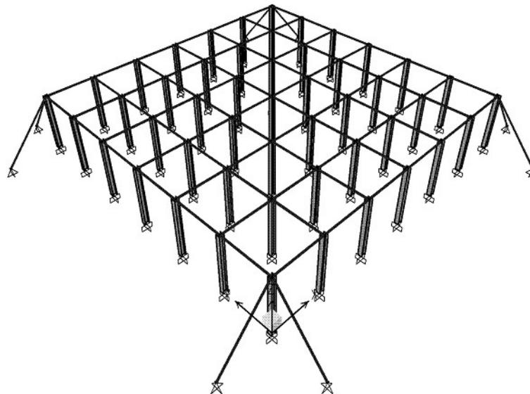
Fig. 3 An overview of structure with external bracing equipped by active of semi-active damping system
