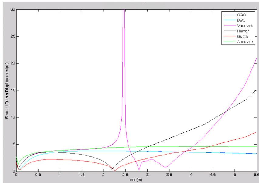
Fig. 8 The curves of lateral displacement in corners which far from eccentricity
