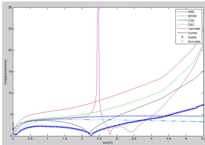
Fig. 5 The lateral displacement relative to structural eccentricity for all methods in the second mode
