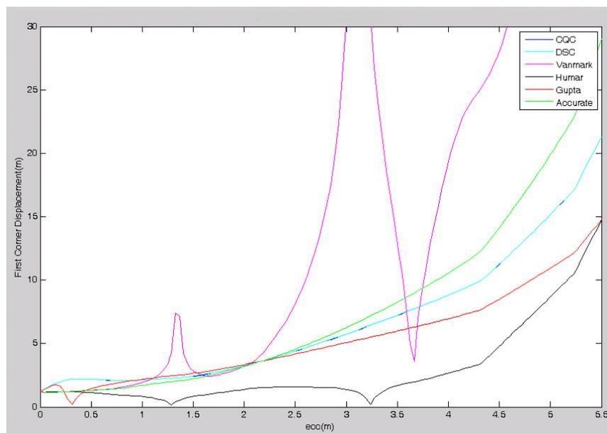
Fig. 7 The curves of lateral displacement in corners which near to eccentricity
