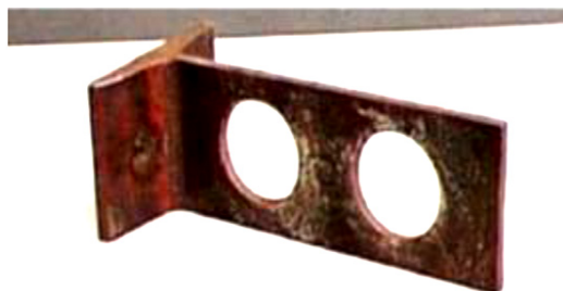
Fig. 3 T-Rib shear connector
