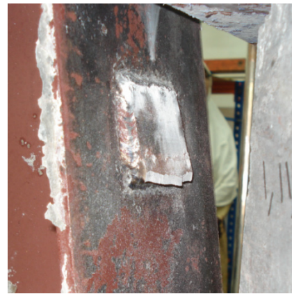
(b) Fractured channel achieved to steel I-Beam
