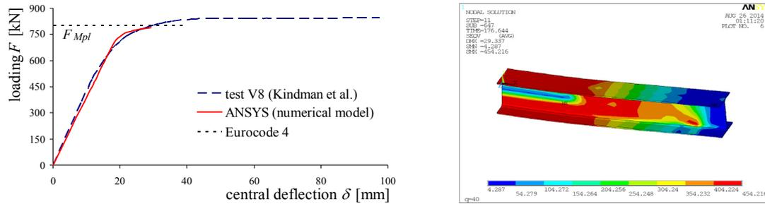
Fig. 11 Load-central deflection relationship (left) and stresses in steel beam (right)
