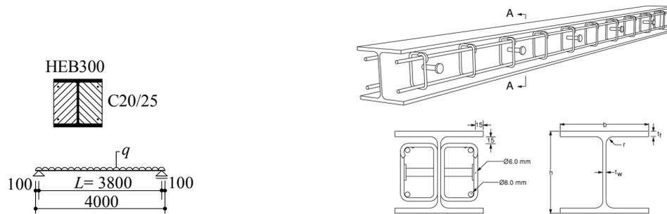
Fig. 8 Studied beam under uniform loading and its steel part
