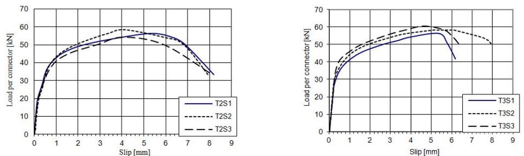
Fig. 5 Load-slip relationship of studs with diameter 13 mm (Series T2 and T3)
