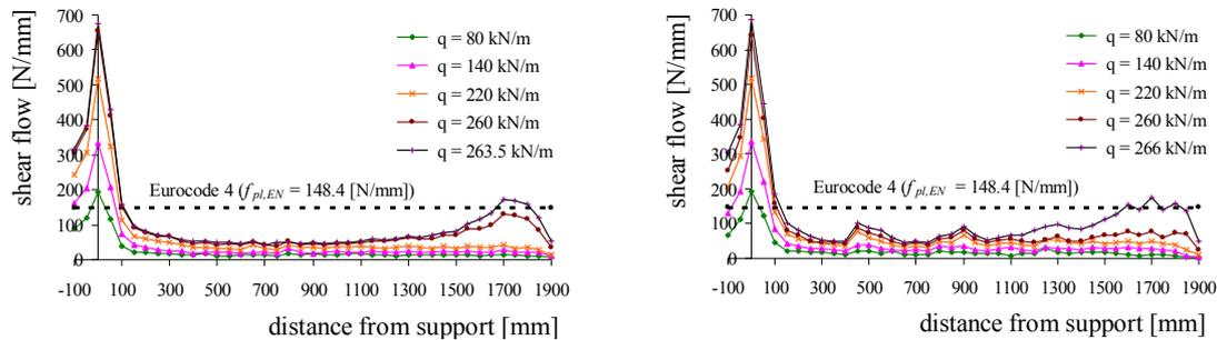
Fig. 15 Shear flow transmitted by friction in steel-concrete contact with friction  $\mu = 0.2$ . Beam without studs (left) and with studs (right)
