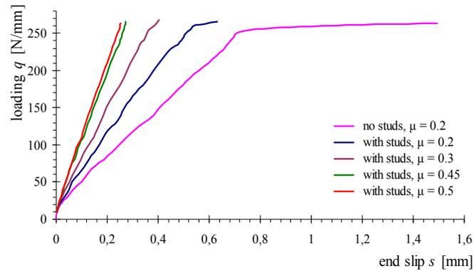
Fig. 13 Load-end slip curves
