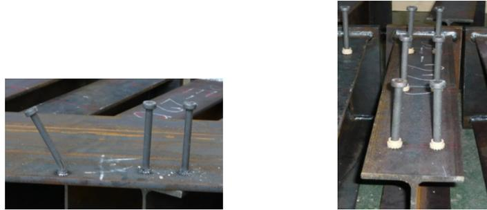
Fig. 2 Standard stud bent test and steel part of specimens with studs
