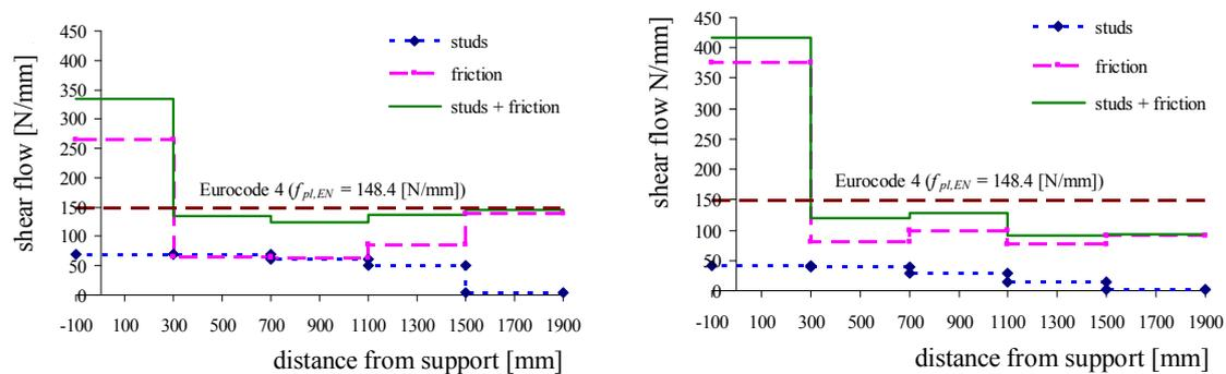
Fig. 16 Longitudinal shear transmitted by studs and due to friction. Friction coefficient  $\mu = 0.2$  (left) and  $\mu = 0.5$  (right)
