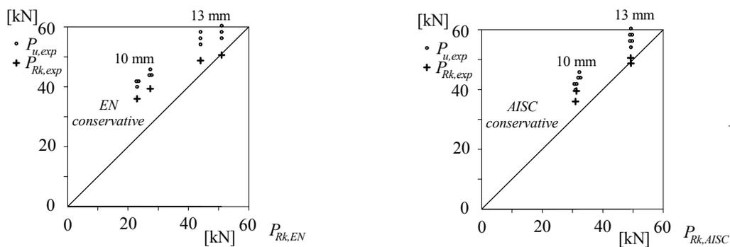
Fig. 7 Comparison of experimental strengths with expressions according to EN 1994-1-1 (2004) and AISC (2010)
