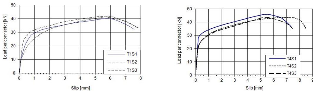
Fig. 4 Load-slip relationship of studs with diameter 10 mm (Series T1 and T4)
