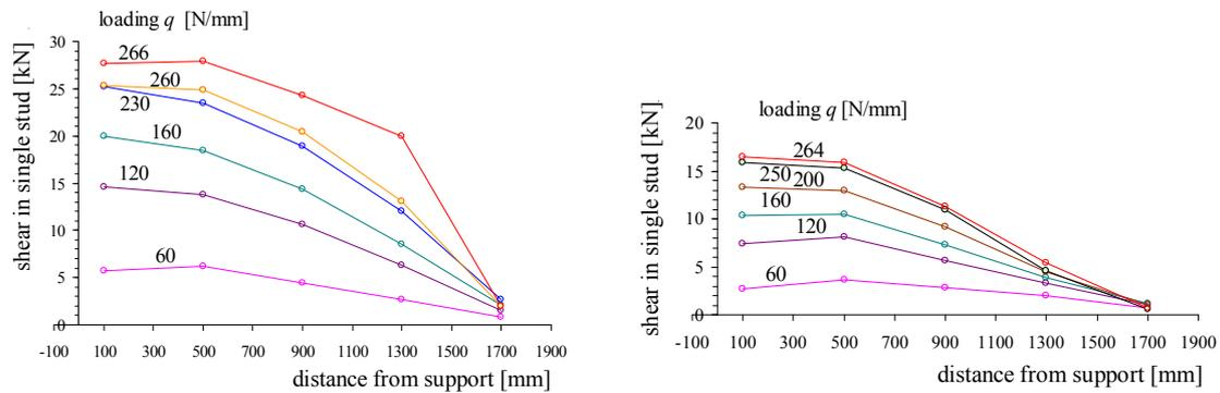
Fig. 14 Shear force in single studs (with the location of studs in curve breaks and spacing of 400 mm). Friction coefficient  $\mu = 0.2$  (left) and  $\mu = 0.5$  (right)
