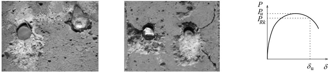
Fig. 6 Typical stud failure traces and evaluation of stud slip capacity
