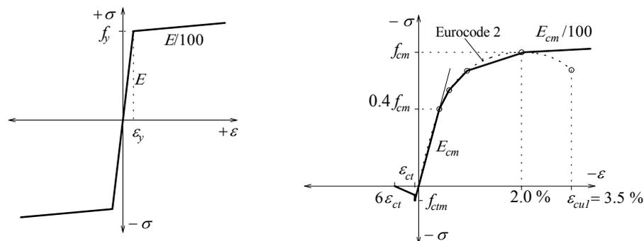
Fig. 9 Nonlinear stress-strain behavior of steel (left) and concrete (right)
