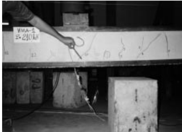
Fig. 8 First test bottom flange weld rupture
