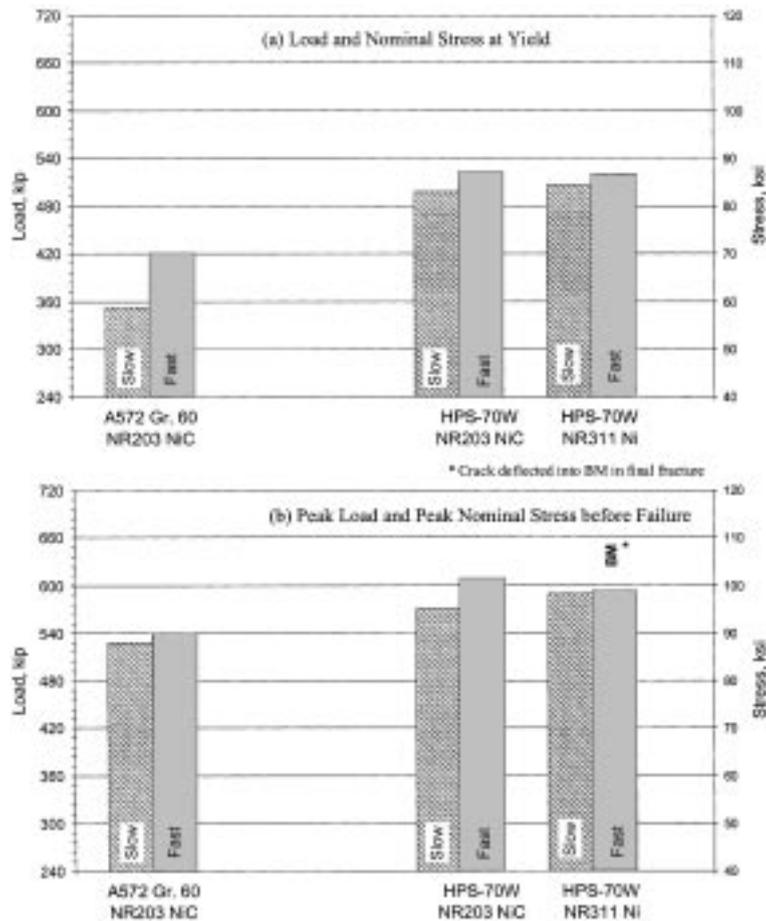
Fig. 12 T-stub test results: (a) load and nominal stress at yield; (b) peak load and peak nominal stress before failure.
