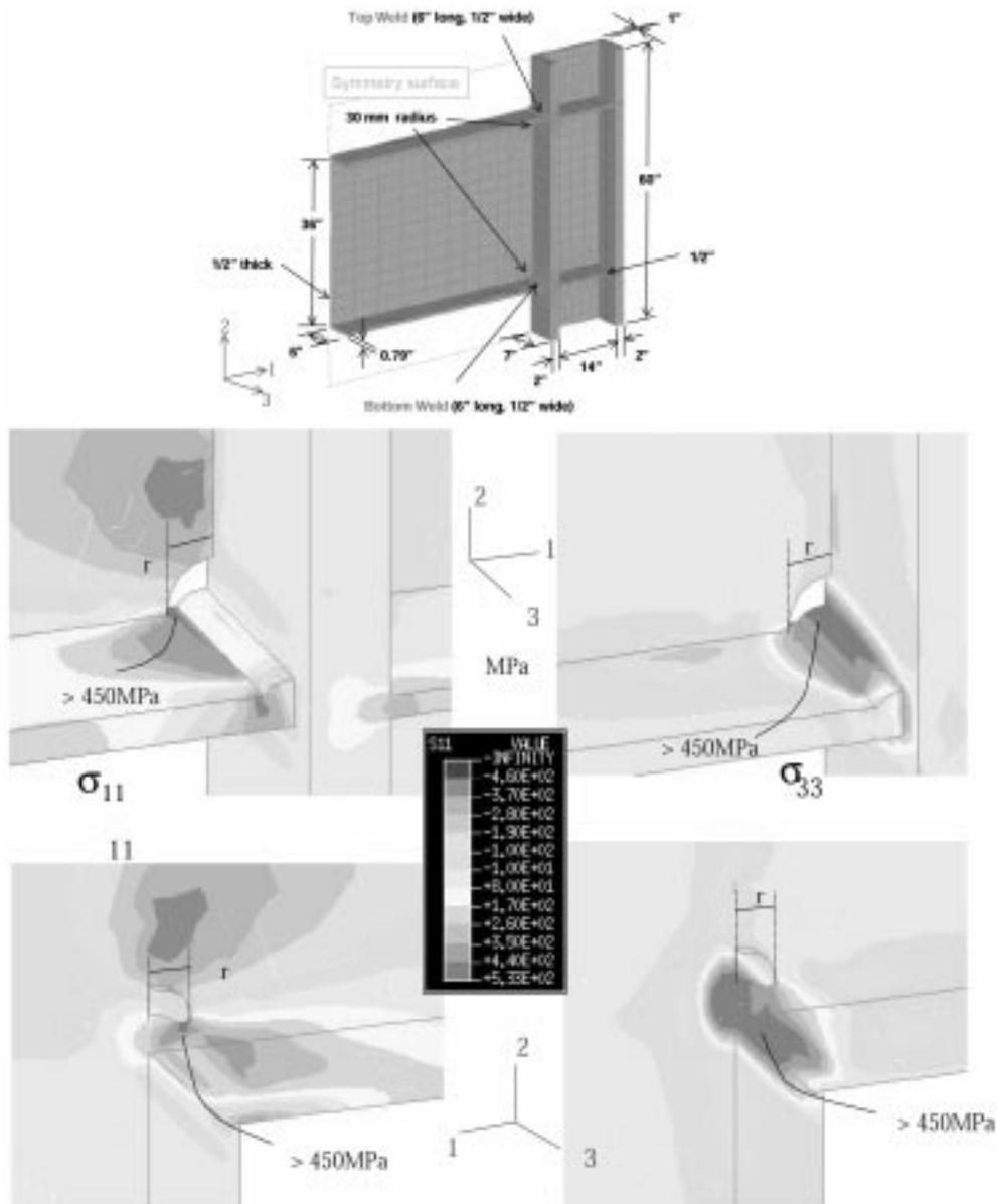
Fig 14. 3D Residual stress distributions in a moment frame joint
