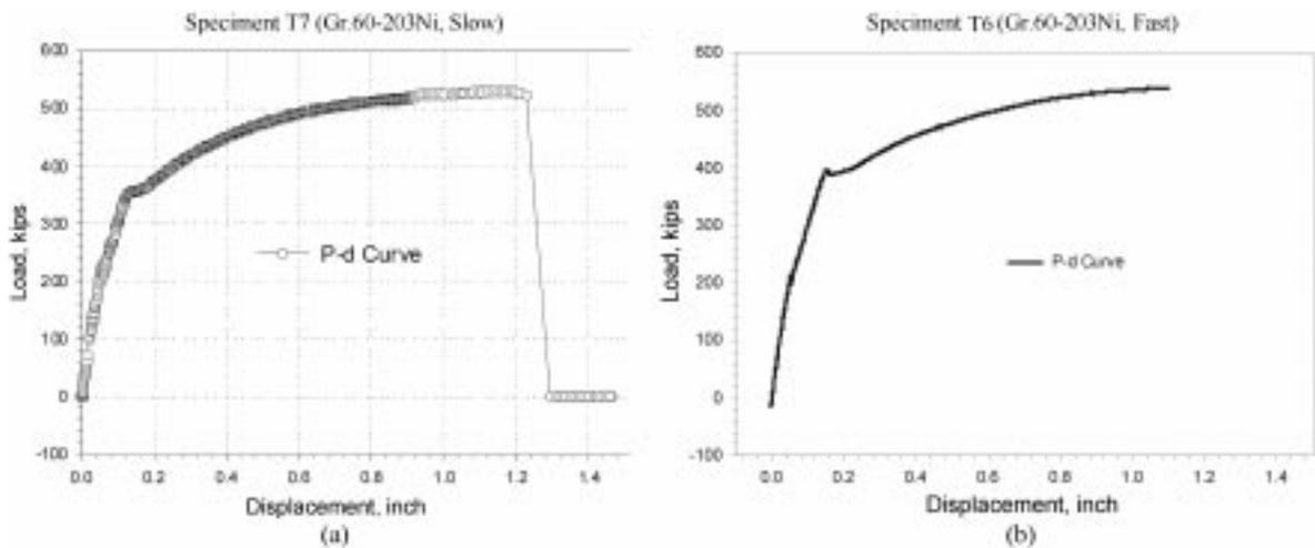
Fig. 8 Measured load-displacement curves for T-stub specimens (BM/WM: A572 Gr. 60/NR203 NiC): (a) Quasi-static loading; (b) Fast loading
