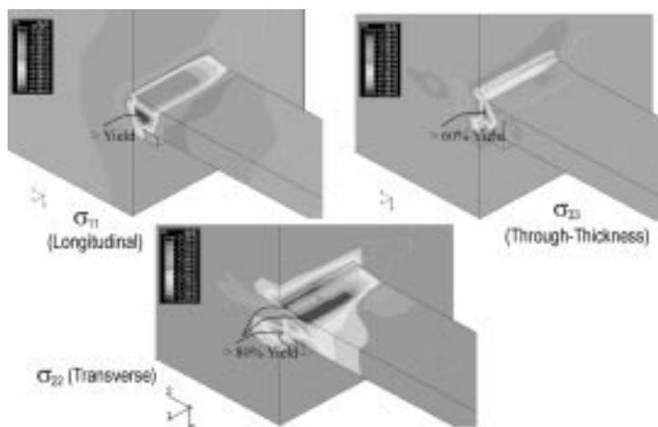
Fig. 10 Predicted residual stress distributions in T-stub specimen
