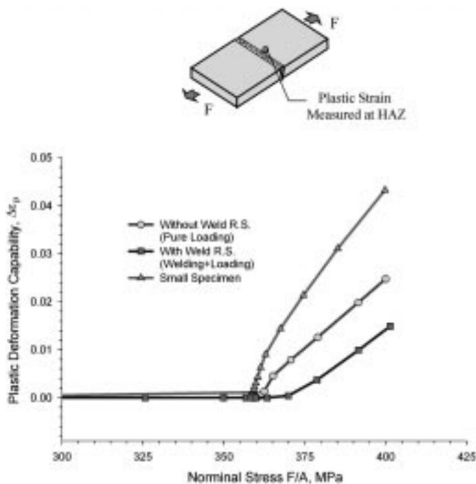
Fig. 3 Local plastic deformation capacity as a function of constraint and welding-induced residual stresses (BM: A36 with matched WM)
