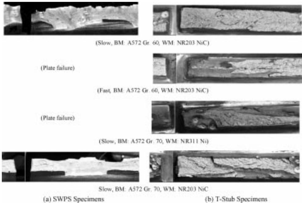
Fig. 13 Comparison of fracture surfaces between SWPS and T-stub specimens for failure in the weld
