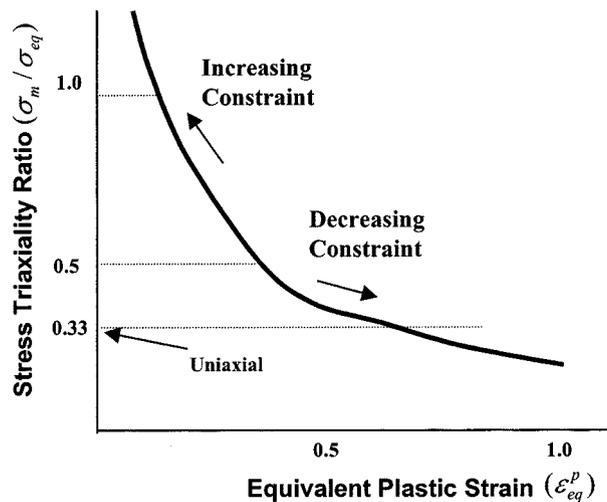
Fig. 1 Typical failure locus for metals as a function of joint constraint
