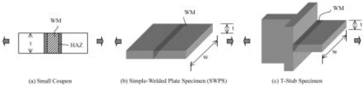
Fig. 2 Typical failure locus for metals as a function of joint constraint: (a) Small coupon-ASTM E8; (b) Wide plate specimens-simple welded plate specimens; (c) T-stub specimen
