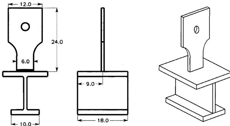
(b) T-Stub Specimen (Unit: mm)
