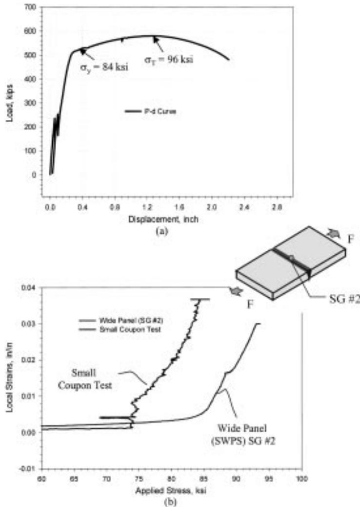
Fig. 6 Sample tensile test results-SWPS (BM: Gr. 70; WM: 311Ni, slow loading): (a) load vs displacement; (b) comparison of local strain development between SWPS and small coupon (E8)
