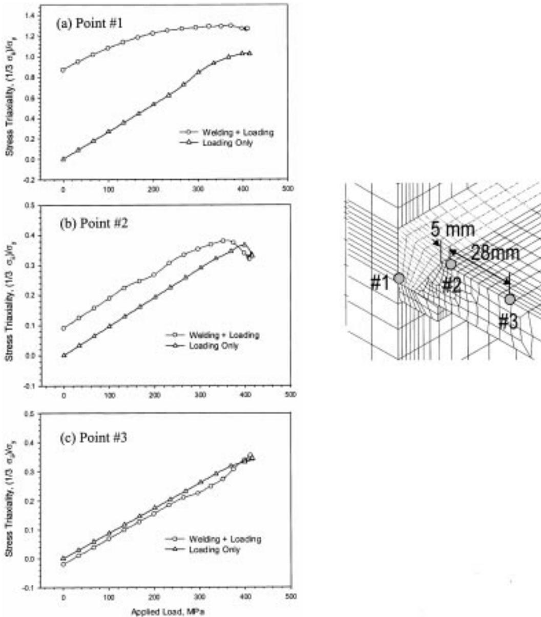
Fig. 11 Stress tri-axiality development in T-stub specimen as a function of remote loading and welding residual stresses: (a) point
