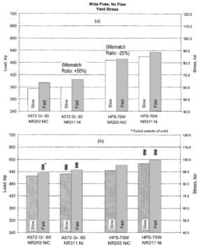
Fig. 7 Wide plate specimen test results: (a) load and nominal stress at yield; (b) peak load and peak nominal stress before failure (Note: BM indicates failure occurred outside of weld in base metal)
