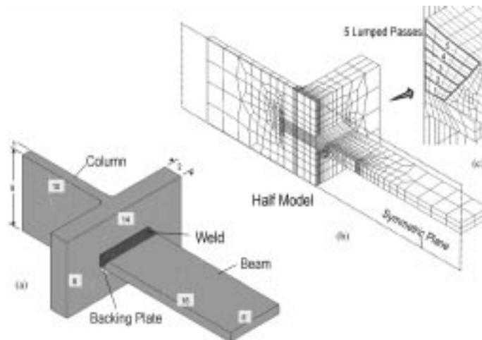
Fig. 9 Weld residual stress model for T-stub specimens: (a) specimen geometry, (b) finite element model, (c) weld pass details
