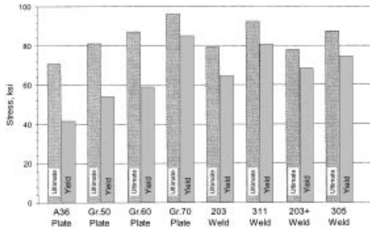
Fig. 5 Summary of small coupon (ASTM E8) test results
