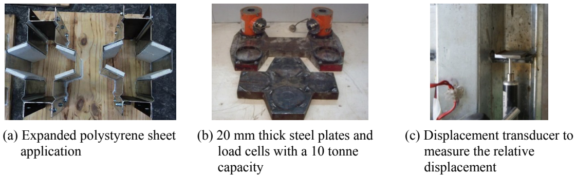
Fig. 9 Details of specimens and measurement equipment
