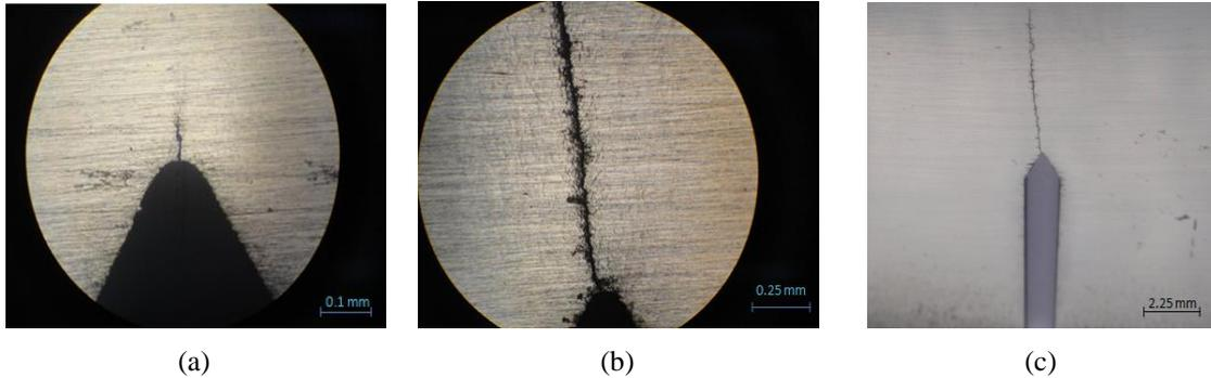
Fig. 10 Microscopic images of the crack at the initial notch at certain cycles. These images are magnified to 25x, 10x, and 1x sizes
