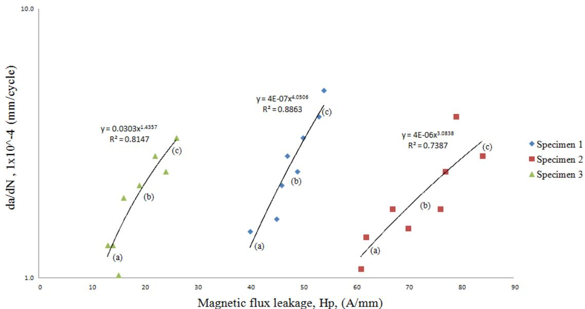
Fig. 11 Correlation between crack growth rate and magnetic flux leakage from the MMM signals
