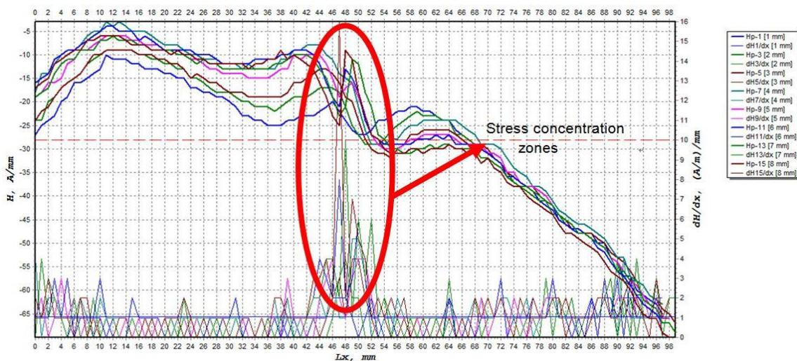
Fig. 7 The amplitude of SMLF signals,  $H_p(y)$  and  $dH/dx$  for specimen 1
