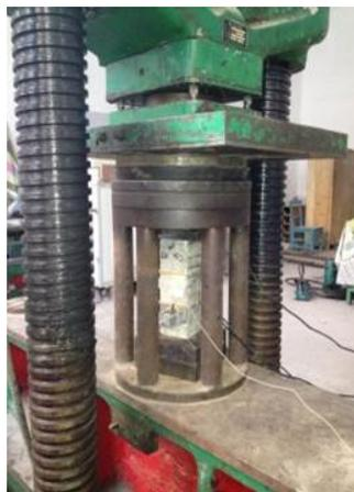
Fig. 1 Testing equipment of concrete compressive strength test
