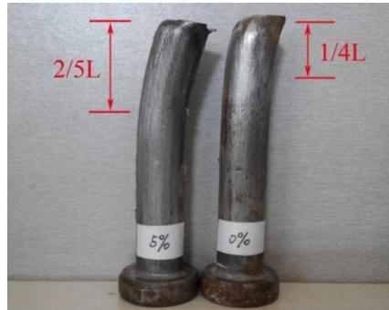
Fig. 12 Deformation of the stud in RRFC and normal concrete
