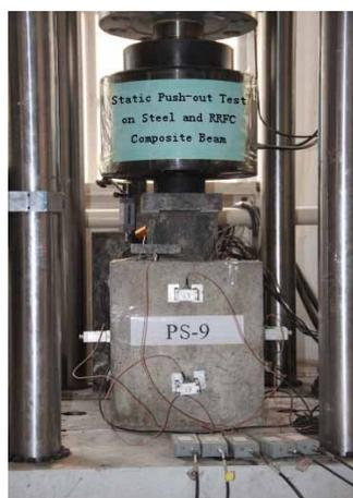
Fig. 6 Loading setup of the push-out test
