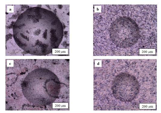
Fig. 6 Response graph for the tensile shear strength g. 6 Brinell hardness traces on (a) the pure Al matrix; (b) AlB<sub>2</sub>/Al composite; (c) Al-Cu matrix; and (d) the AlB<sub>2</sub>/Al-Cu composite
