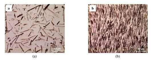
Fig. 3 Microstructure of (a) the as-cat master Al-B alloy; and (b) AlB<sub>2</sub>/Al composite material after filtration
