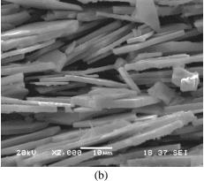
Fig. 5 SEM image of the deep etched: (a) as cast Al–B alloy before filtration; and (b) AlB<sub>2</sub>/Al composite after filtration
