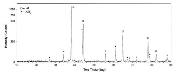
Fig. 4 The XRD spectra of the Al-B alloy
