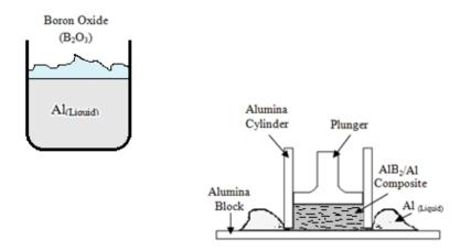
Fig. 2 The production scheme of the composite materials: (a) reaction melted aluminum with  $B_2O_3$  at 1300°C, structures; and (c) increase the AlB<sub>2</sub> boride concentration by the filtration system at 700°C
