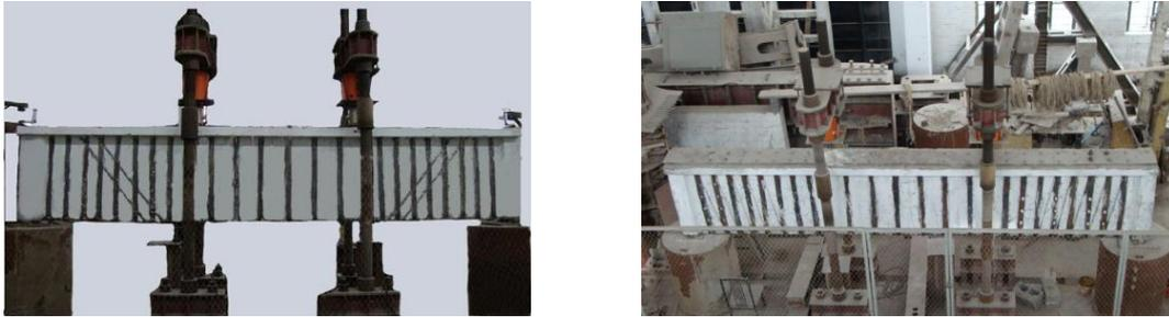
Fig. 11 Test setup for CBSP-strengthened beam
