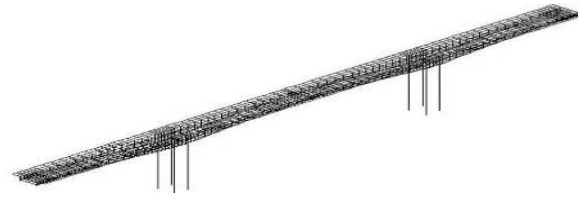
Fig. 7 Spatial grid model of large-span concrete box beam bridge with continuous rigid frame
