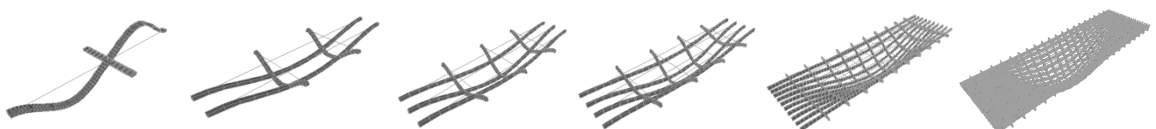
Fig. 11 Typical first mode shape of grid systems ( L_1/L_2 = 3.0 ), Fixed
