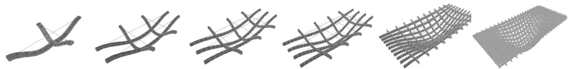
Fig. 8 Typical first mode shape of grid systems ( L_1/L_2 = 2.0 ), Fixed
